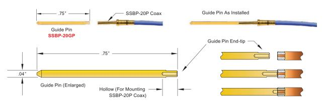
Inserting Guide Pin into the End of SSBP-20P Coax
