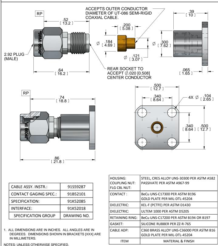
DATE APRVD. DATE TITLE 2.92 PLUG (M) 4 HOLE REAR MOUNT RE\ RELEASED PLC 07/09/12 07/09/12 A FLANGE CABLE CONNECTOR Southwest Microwave, Inc. ACCEPTS .086 SEMI-RIGID CABLE 9055 South McKemy Street DATE: 9/7/11 DRN BY: MODEL NO. REV. Tempe, Arizona 85284-2946 EJO 1001-11SF SOUTHWEST Telephone (480) 783-0201 SCALE: 3:1 А **MICROWAVE** Fax (480) 783-0360 DWG. NO. SHEET: 1 OF 1 79K60678
