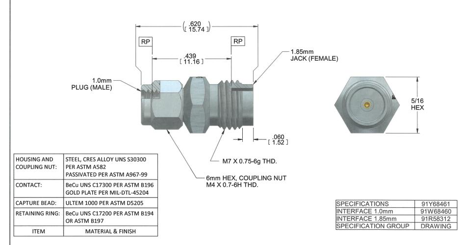
1. ALL DIMENSIONS ARE IN INCHES. ALL ANGLES ARE IN DEGREES. DIMENSIONS SHOWN IN BRACKETS [XXX] ARE IN MILLIMETERS.
