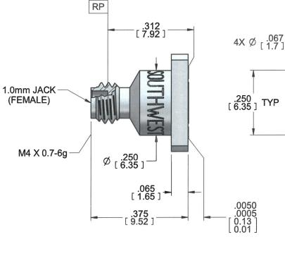
$\emptyset$  [  $\stackrel{.029}{0.74}$  ] RAISED METAL **CONTACT RING** (360° SURFACE CONTACT) ACCEPTS Ø.005/.006 PIN MAXIMUM PIN DEPTH .035
