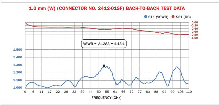
VSWR =  $\sqrt{1.283}$  = 1.13:1 maximum for each connector, as shown. Contact Southwest Microwave for performance specifications for all other 1.0 mm (W) connectors.
