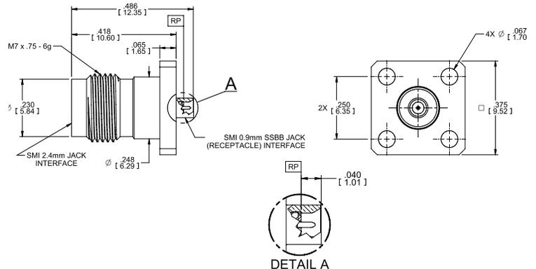
Southwest Microwave SuperMini Board-to-Board Connector solutions maximize electrical performance of the transmission path between connector and circuit while accommodating axial misalignment of 10 mils and radial misalignment of +/- 10 degrees with no resonance.
