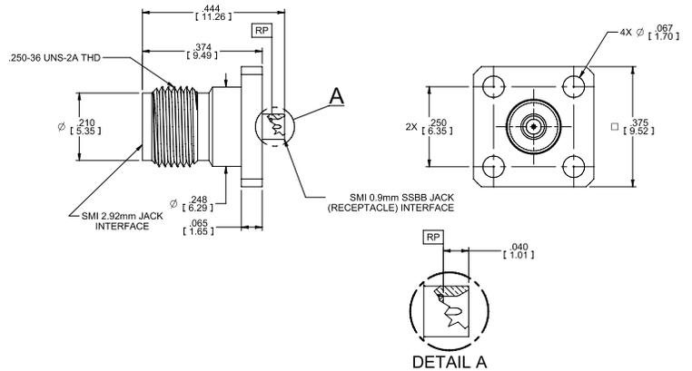
**SSBB SIZE 20 HERMETIC JACK TO 2.92 mm JACK 4-HOLE .375 SQUARE FLANGE (18 GHz)**
