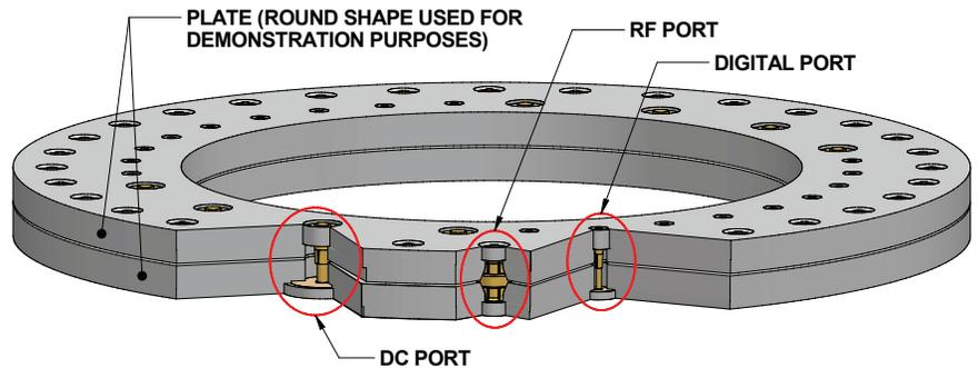
Cross-section view of custom design. Southwest Microwave SSBB RF connectors can be built onto any plate shape with DC and digital ports.
