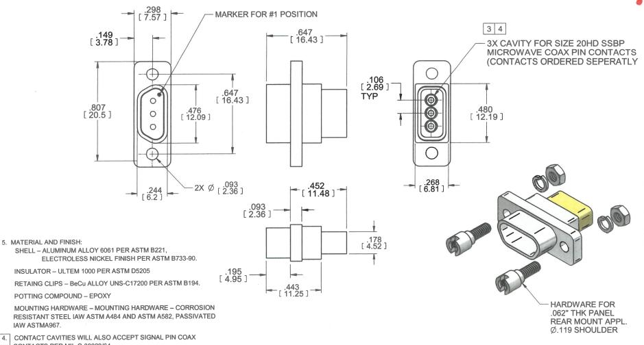
4. CONTACT CAVITIES WILL ALSO ACCEPT SIGNAL PIN COAX CONTACTS PER MIL-C-39029/64.
