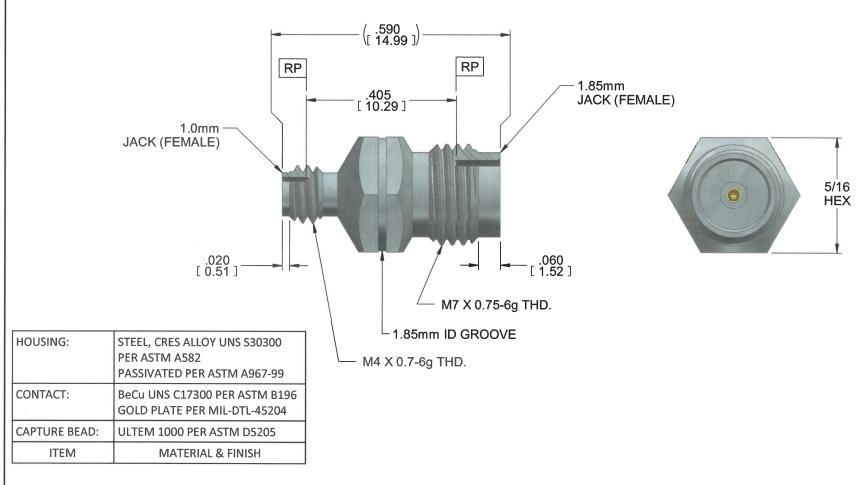
ALL DIMENSIONS ARE IN INCHES. ALL ANGLES ARE IN DEGREES. DIMENSIONS SHOWN IN BRACKETS [XXX] ARE IN MILLIMETERS.
