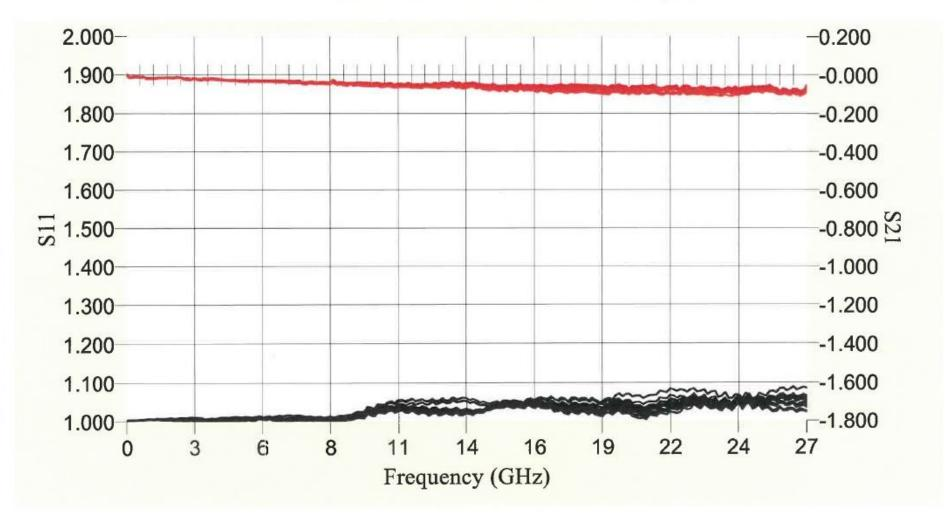
Operator Ann Date 10-22-2019 @ 08:26:47 Model number: 232-502SF QCIR:110304-000; Serial number 9 File name 9.dat Measurements,1,2,3,4,5,6,7,8,9,10,11,12,13,14,15,16 Notes SMA J TO SMA J ADP SOLT
