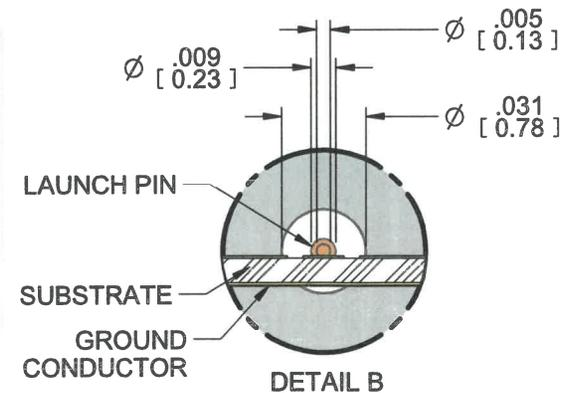
1. ALL DIMENSIONS ARE IN INCHES. ALL ANGLES ARE IN DEGREES. DIMENSIONS SHOWN IN BRACKETS [XXX] ARE IN MILLIMETERS.
